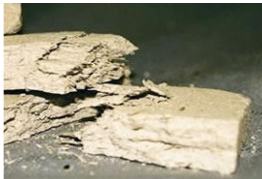
Pieces of Asbestos Insulating Council (AIB)
